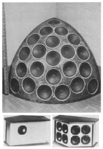
An ideal pulsating sphere is simulated by 4he eighth of a sphere shown at upper left. The eighth sphere in a corner of a room is equivalent to a full sphere floating in empty space, since ideai walls are to sound as ideai mirrors would be to
