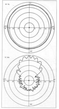
fig: The radiation patterns, at a low frequency (top graph) and a high frequency (bottom graph), of a loudspeaker in an anechoic ahamber. Six dB difference between two measurements corresponds to a doubling of sound pressure. At 15 kHz, the pressure radiated forward (at 0°) averages about 25 times greater than pressure radiated 60° or more off axis. At 50 Hz, however, pressure is much closer to equal in ali directions, off by only about 30 per cent even behind the speaker.
